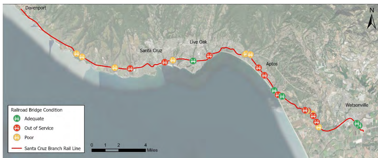
Figure 3 - Condition of Railroad Bridges along the SCBRL
