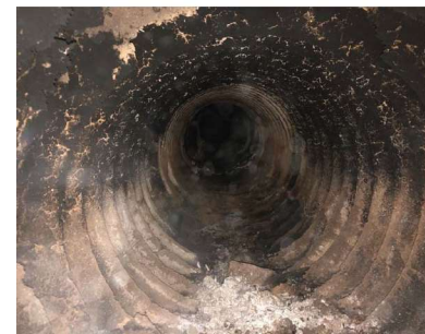
Inside of pipe showing corrugations from melted culvert
